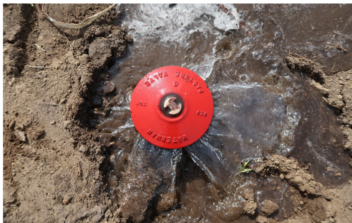
Figure 4. Alfalfa riser gives more control over flood irrigation
